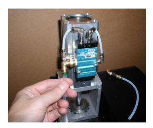
8. Pump is ready to run when the system is up to operating temperature. The air pressure may have to be readjusted to obtain desired glue pressure.
