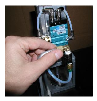
7. In some cases the melter may Teflon tubing connected to the pump rather than rigid piping. If this is the case, you need only remove the tubing and fitting that came with the replacement pump (shown laying to the right below), and connect the tubing on the melter directly to the pump as shown below.
