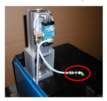
5. Install the hardware end of the assembly (circled in the picture immediately above) to the air tube on the unit as shown below. **Do Not Allow the Teflon Tube to Kink.**
